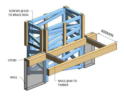
SECURE KIRKYL FRAME TO ROOF STRUCTURE AT CEILING LEVEL
